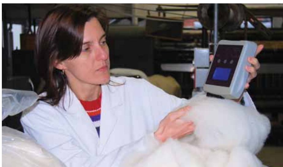
AgResearch Textile Science & Technology Section Technician Mihaela Hnat with the Verifi TT hand-held reader that gives textile traceability by detecting a unique 'signature' in yarn, fabric or carpet.
